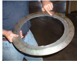
7. Install 4 to 8 bolts depending on flange size to align flange. Use a  $\frac{3}{4}$  drive impact to tighten, not exceeding 30% of final torque. Check flange gap for parallelism.
