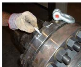
**12. Step-1** Apply 50% of the maximum torque to 30% of the total bolts in a pattern
