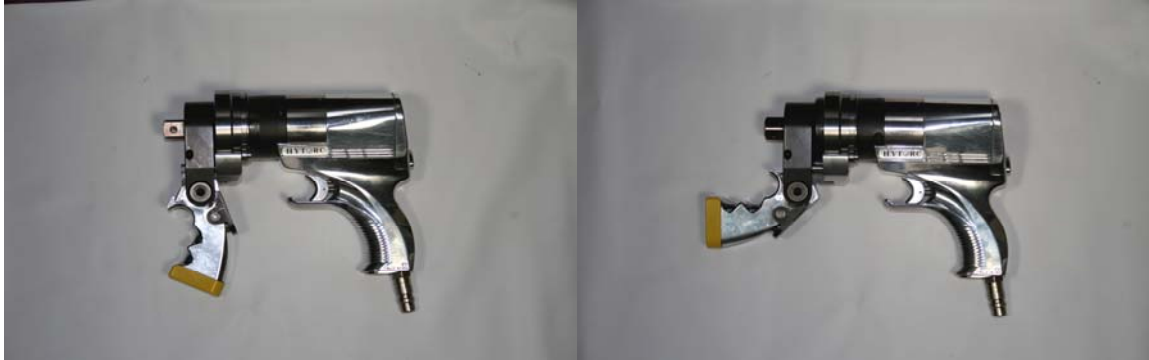
Figure 4: Torque Operation Settings- High Speed (Left) and Maximum Torque (Right)
