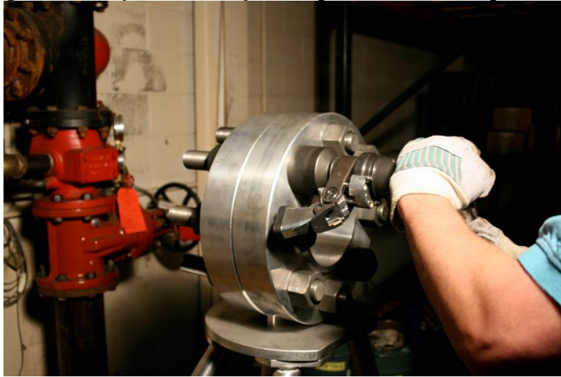
Figure 6: Safety Position for jGun Flip in Maximum Torque Setting
